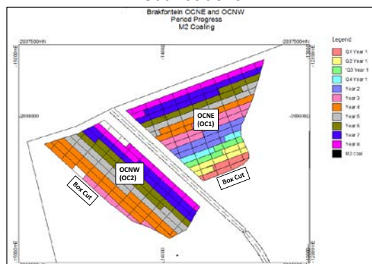
Figure 3-4: Brakfontein Mining Layout with Box Cut Positions
