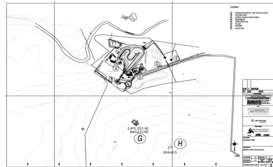
Figure 1-14: NCC Diepspruit Resource Underground Mine Surface Layout
